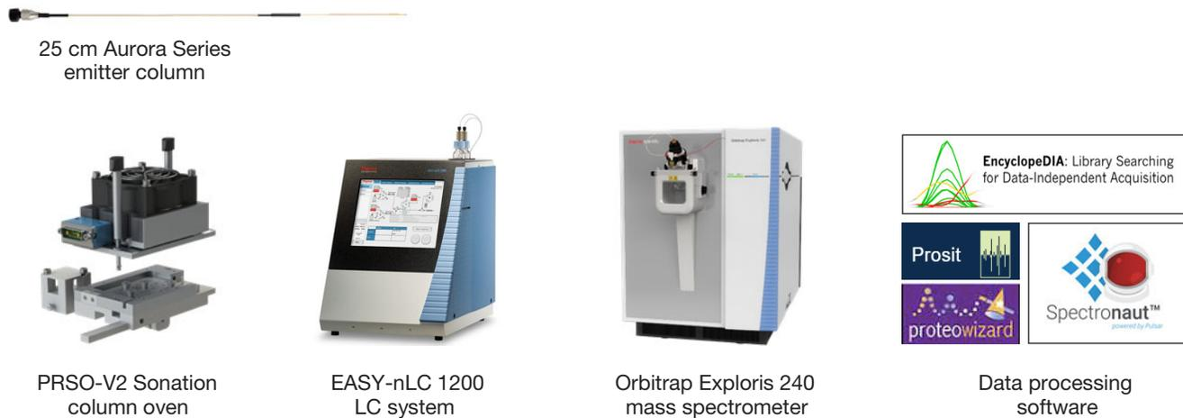
Figure 1. LC-MS setup for DIA performance evaluation
